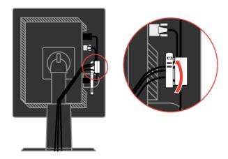
Wrap the Cable Wrapper around the cables.
